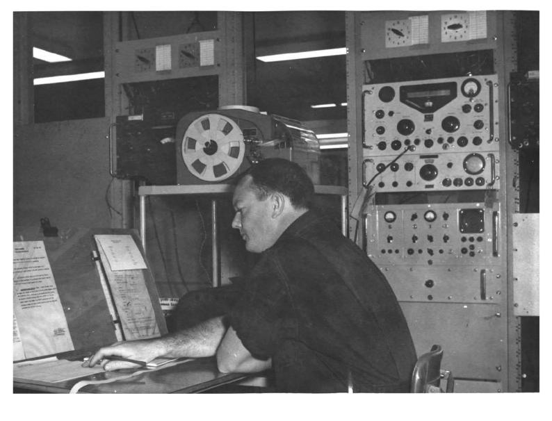
pictured here (from top) consists of co-axial aerial switching, RACAL RA-17C receiver, sideband adaptor and TFS-3 convertor. The reperforator above the operator's head is a T-Lock15 which is cutting a 5 unit chadded tape for EDP processing.
