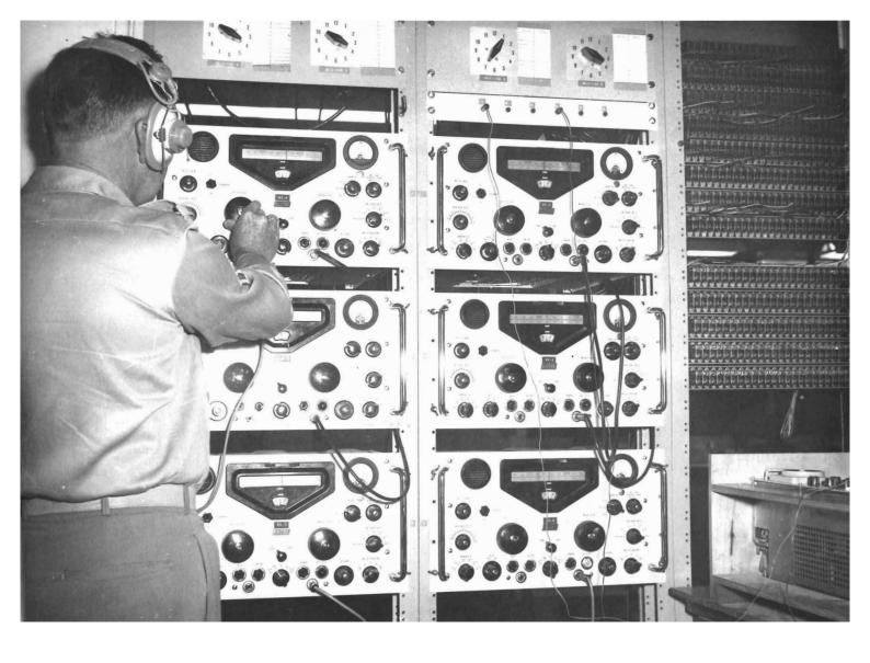
This photograph depicts the machine intercept receiving bay where six RACAL RA-17C receivers are used in conjunction with ELMUX multiplex equipment. The output of each receiver is coupled to drive a frequency shift converter which in turn is coupled to the ELMUX consoles. 18 separate telegraphic channels are currently monitored on this position but the equipment is capable of handling 24 full telegraphic channels.
