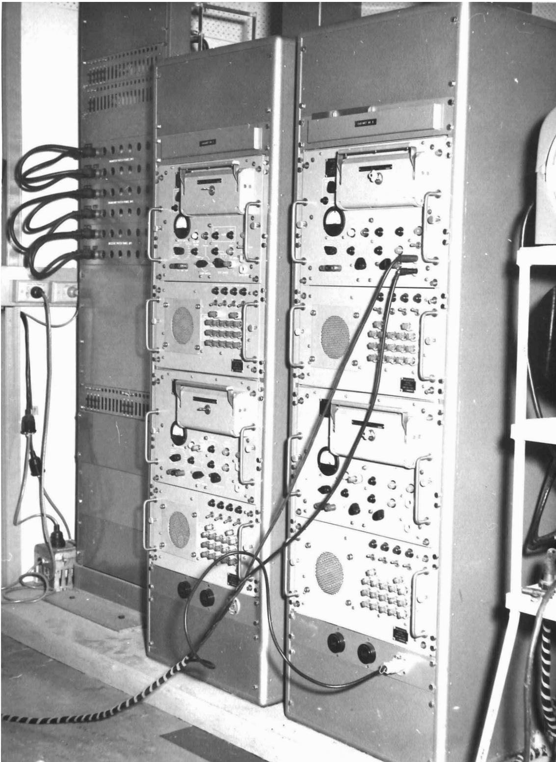
This photograph, taken in the communications room shows two KW-26 crypto consoles which terminate the 3TEIJ-DSD communications line. 24 hours per day direct communication is maintained with DSD. Over three quarters of a million groups are currently sent and slightly less than this total received monthly on this link.
