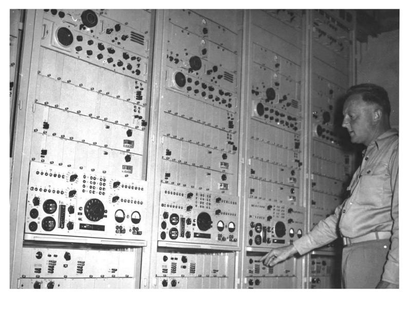
Pictured here are four of six ELMUX multi-channel demodulation systems which occupy the southern end of the main set room. Operator in attendance
